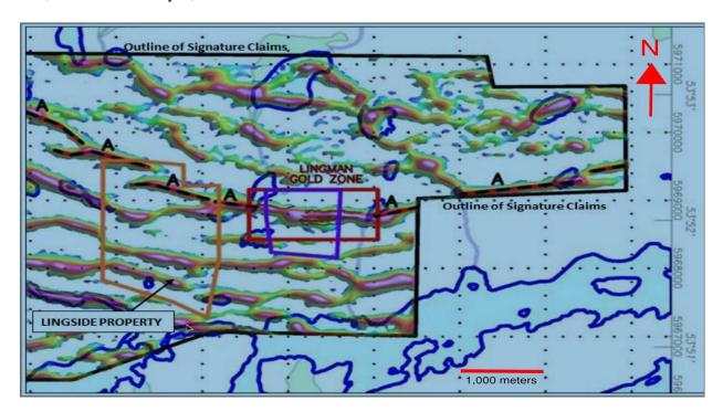
Airborne geophysical results of VLF-EM highs and conductor axes on the Lingside and Lingman Lake properties. Conductor highs are in red and conductor axes linears are black, "A"s are high priority segments. For more information, see the Company's press release dated May 2, 2018, entitled "Gold mineralized zones at Signature's Lingman Lake Property respond to geophysical survey".
