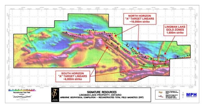
Target classification definition: Target ranking is defined by correlation of Magnetic and VLF characteristics with the known gold zones at Lingman Lake. Hence, an 'A' target has the strongest correlation, followed by 'B' and 'C'. We fully anticipate lower ranking targets to be identified as interpretation is on-going.
